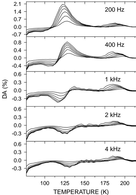
Fig. 2. Isochronal relaxation spectra of the YIG sample sintered in  $\text{CO}_2$  at  $1450^\circ\text{C}$  at different measurement frequencies.
