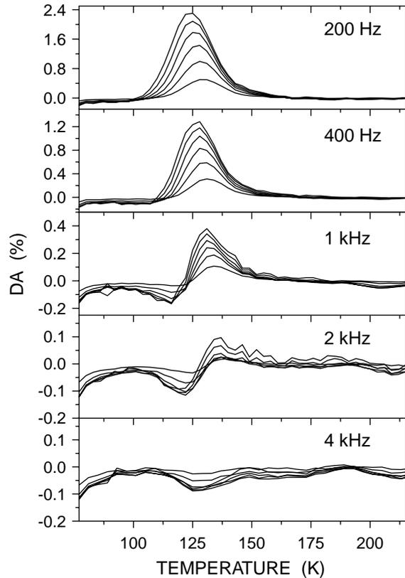
Fig. 1. Isochronal relaxation spectra of the YIG sample sintered in  $\text{CO}_2$  at  $1420^\circ\text{C}$  at different measurement frequencies.
